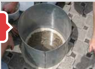
Adequate measurements of infiltration can be obtained with a single ring infiltrometer.
