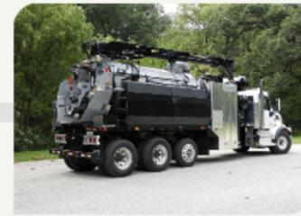
2019 - Vactor introduces TRUVAC, a brand of premium vacuum excavator trucks satisfying safe-digging requirements for locating and verifying underground utility lines and pipes.
