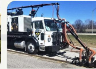
2023 - Federal Signal acquires Blasters Inc., a manufacturer of truck-mounted waterblasting equipment, with applications in road-way projects, airport runway rubber and marking removal and other surface preparation projects.
